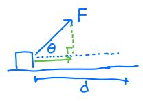
If F is not parallel to d, we need the component of F in the direction of d. So the green arrow is Fcoso and is the part of F that is in the direction of d.
